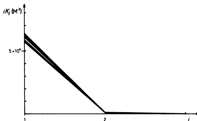
Fig. 2. Klotz affinity profiles for binding of ceftriaxone to human serum albumin. The meaning of this plot is explained in Ref. 21. Thirty acceptable values of the first stoichiometric binding constant are plotted on the ordinate indicating the variation within a probability limit of 0.75. Two times the second stoichiometric binding constant is likewise shown at the abscissa value of 2.
